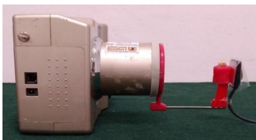
Fig 1: The tooth positioning assembly to standardize the distance and position the tooth preoperatively and postoperatively at same distance.
