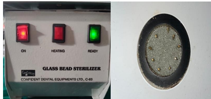
Figure depicting placement of the rotary endodontic files at the periphery of the glass bead sterilizer.
